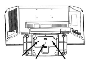
**Note**: Lock the screw middle first, then the others, to avoid holes aiming incorrectly
